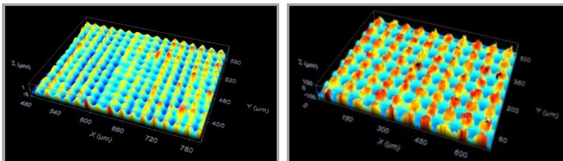
Figure 2: Pyramidal structure obtained by picoseconds laser and grid lines obtained by nanoseconds laser.
