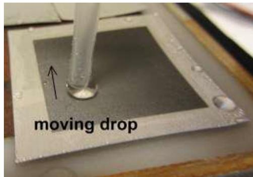
Figure 6: Micro-structured sample (Coating 6) tested under condensation conditions
