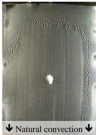
Figure 8: Aluminium plate with coating 3, 10 x 15 cm, hold at  $-4^{\circ}\text{C}$  for 20 min after placing ice in the middle. Environment  $+12^{\circ}\text{C}$ ,  $\sim 90\%$  relative humidity, continuous condensation.
