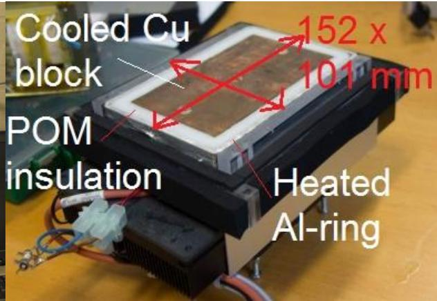
Figure 4: Cooling block for the ice test chamber.
