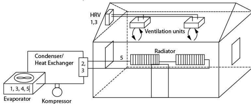
Figure 1: Schematic of a building with heat pump and heat recovery ventilation.
