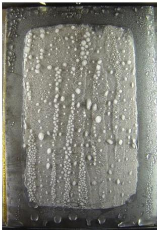
Figure 7: Bare aluminium plate with a frost layer hold at  $-0.5^{\circ}\text{C}$  for 15 min to verify contact with the cooling block. The edge is heated and thus ice free.
